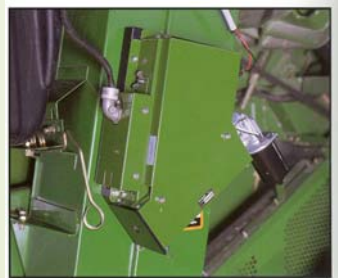
Elevator Mount Moisture Sensor
